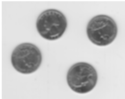
Filtered Image with Border Replication
